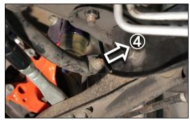
Remove the 4 bolts/nuts for both the left and right side of the stabilizer bar. (Right side shown above) \*\* Removing the stabilizer bar ensures sufficient clearance for the oil pan to be lowered and removed. \*\* A modified 240SX may look slightly different but fundamentally the same components will need to be removed.
