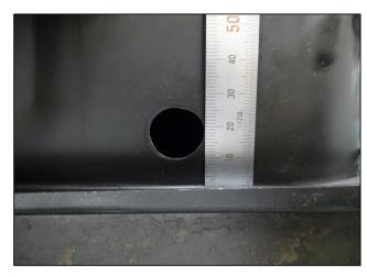
Vertically, the hole center should be 18mm from the oil pan flange.
