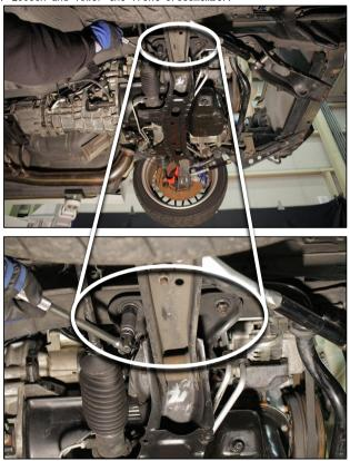
Loosen the 4 bolts/nuts holding the front crossmember in place. (left side x2, right side x2)  $\times$  Do <u>not completely remove</u> the bolts/nuts during this process.
