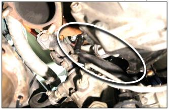
2. Cut the OIL PROOF HOSE to the appropriate length and connect onto OIL DRAIN PIPE B (from step 4.3.) and secure using the included HOSE BAND.
