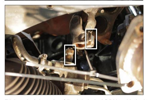
With the steering wheel centered, carefully mark the sheering shaft U-joint position in relation to the steering rack pinion gear this is to ensure correct steering alignment upon reinstall.
