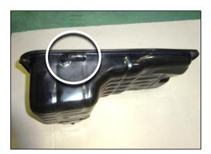
The OIL DRAIN PIPE B should be installed parallel to the oil pan flange.
