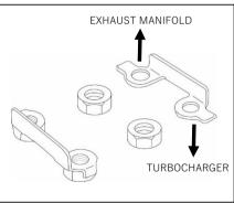
\* After tightening down the lock plates, bend the tabs to secure into position.
