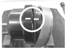
Make note of the alignment of the upper case in relation to the lower case.
