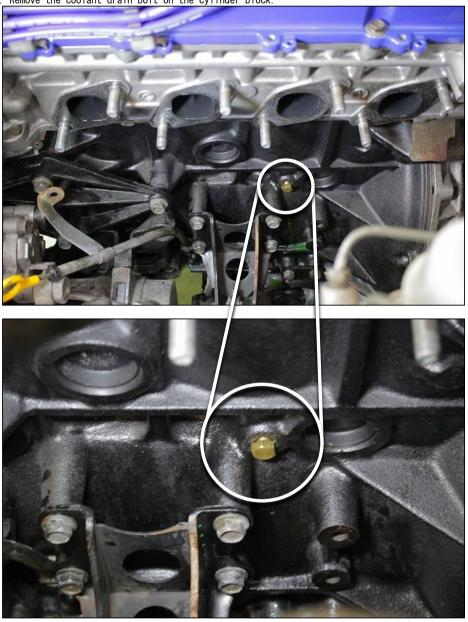
$\ensuremath{\mathbb{X}}$  This hole will later be used for the turbocharger WATER IN FITTING.
