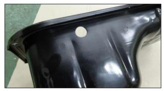
Start with a smaller drill size first (10mm), then expand the hole to 16.5mm.
