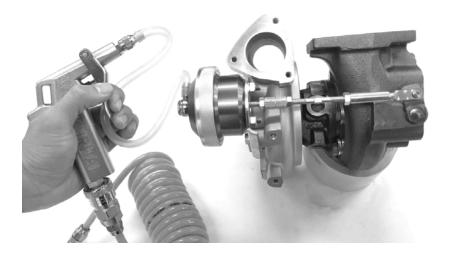
⑤ Apply air pressure to the actuator using slightly higher pressure than the configured springs. This will move the actuator rod, allowing you to reconnect it to the wastegate bracket.
