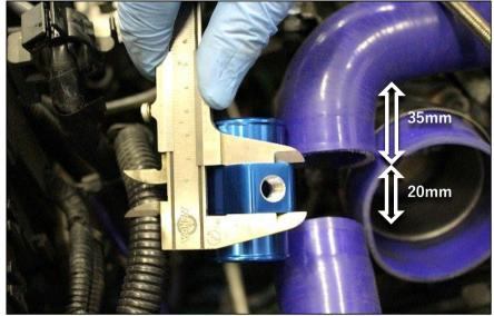
3. Install the WATER PIPE ADAPTER using the included HOSE BANDs.
