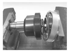
③ Using step 2-1 as reference, clamp and compress the actuator springs in the housing using a vice, then secure using the lock ring.
