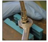
2. Using the included WATER BOLT and WASHERs, attach the BANJO FITTING and MESH HOSE to the turbocharger.
