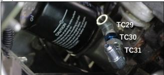
4. Install the oil pressure sensor onto the 3 WAY ADAPTER and reconnect the sensor coupler.
