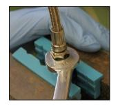
2. Using the included WATER BOLT and WASHERs, attach the BANJO FITTING and MESH HOSE to the turbocharger.
