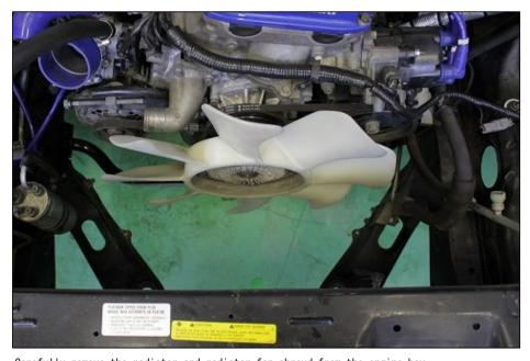
Carefully remove the radiator and radiator fan shroud from the engine bay.
