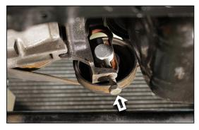
Loosen the center bolt on the AC idler tension pulley, then relieve the tension on the belt to unmount it from the pulley.
