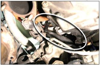
2. Cut the OIL PROOF HOSE to the appropriate length and connect onto OIL DRAIN PIPE B (from step 4.3.) and secure using the included HOSE BAND.
