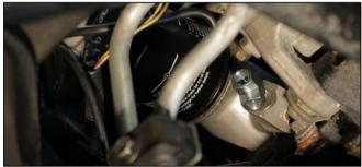
3. Combine the PT 1/8 4AN and  $90^{\circ}$  fitting adapters and install onto the 3 WAY ADAPTER as shown below.
