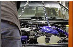
Ensure you have appropriate engine slingers attached to the cylinder head then hoist the engine just enough so that the LH engine mount bracket and bolts can be removed.
