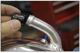
Install INTAKE PIPE A onto the throttle body and pass the opposite end through the opening in the battery tray.
