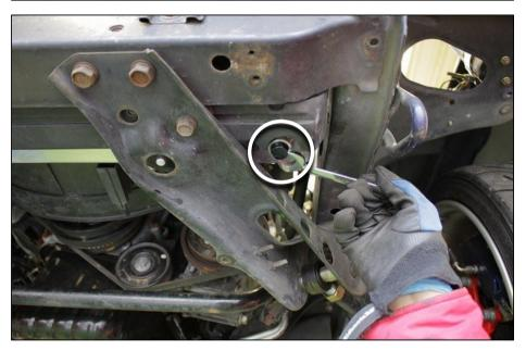
Remove the drain plug on both the oil pan and radiator to drain the engine oil and coolant.
