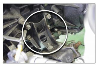
With the engine hoisted, carefully remove the LH engine mount bracket.
