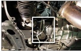
\* The gussets need to be removed so that the oil pan can be detached.
