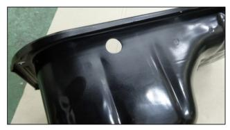
Start with a smaller drill size first (10mm), then expand the hole to 16.5mm.
