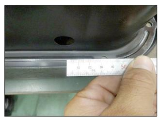
Horizontally, the hole center should be 33mm from the bolt hole center pictured left.
