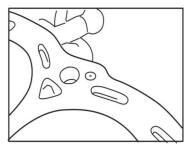
$\Phi$ 1.5mm restrictor installed.
