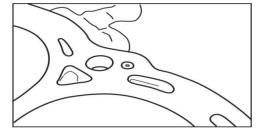
② Using a 5mm pin punch, depress the stock oil restrictor by 6mm.
