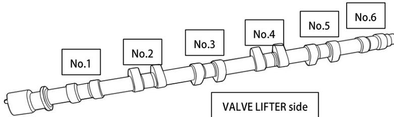
Be careful not to over tighten the cam cap bolts on lobes #1, #2, #4 and #6. Whilst these are easier to tighten than lobes #3 and #5, doing so will result in uneven vertical force, causing the camshaft to warp or even break.
