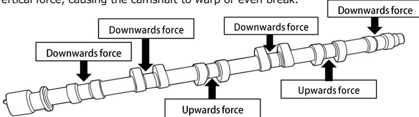
When installing the camshafts, ensure that you tighten down the bolts slowly and evenly so that the camshaft sits level in the cylinder head. To do this, tighten each bolt 180 degrees at a time, starting with a lobe that is already facing the lifter. As you alternate between the bolts with every 180 degree turn, the camshaft should gradually nest into the correct position.
