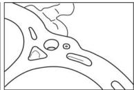
② Use a 5mm pin punch tool to install the stock orifice 6mm deep.
