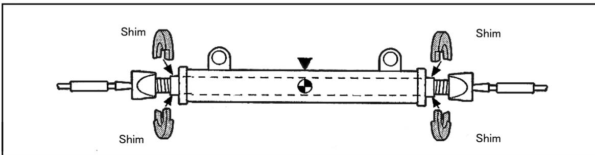
③ Secure the Shims in place with the screws.
