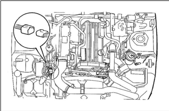
① Remove the Solenoid Valve Connector.
