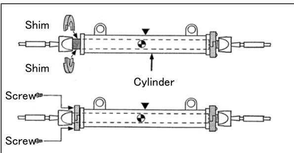
④ Separate the Shims to install them in place.
