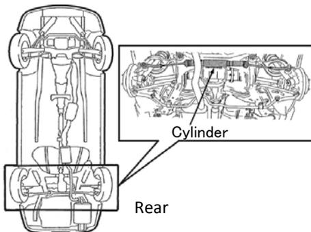
You'll be working on the rear wheels. Check the positions of the cylinders, etc.
