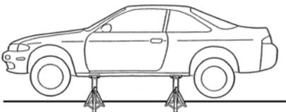
Have the vehicle setup so you can work under the vehicle.
