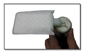
Install the Fuel Pump Filter to the Fuel Pump by using the clip.
