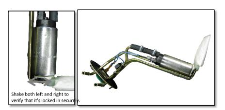
Again, verify that the fuel pump is locked in, secured in it's position. Then install the pump unit back into the fuel tank.
