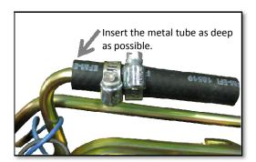
Insert the fuel pump hose inner pipe.
