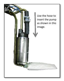
Fit the mount bush on the pump before connecting the fuel hose. Securely insert the mount bush into it's specified position. To securely lock the pump into position, use the fuel pump's body and the bracket to secure it in place during installation.
