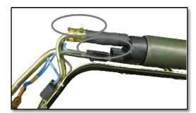
Remove the fuel hose clamp and coupler from the fuel hose.
