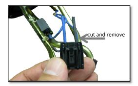
To leave the fuel pump harness as long as possible, cut it around the joint of the coupler.
