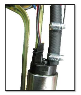
Tighten the hose clamp securely, then connect the coupler to the  $\mbox{\sc Pump}.$
