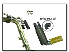
Remove the hose from the Fuel Pump unit. This mounting bush that gets removed will be reused. So please don't lose it.
