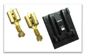
Disconnect the stock harness from the Fuel Pump. Then cut the end off and connect the coupler (included).
