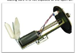
Remove the fuel pump from the fuel tank. Carefully secure the float in the tank, making sure not to damage it.
