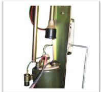
Be sure to pull it out straight because the Fuel Pump is plugged into the pipe Bracket.
