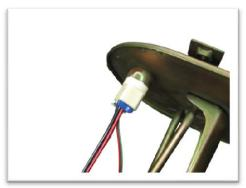
Make sure that the Insulator is firmly positioned at the bottom of the Fuel Pump. Then tighten the Hose Band.
