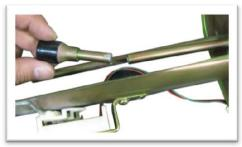
Have the Fuel Pump assembled with the washer and insulator that was supplied with the Fuel Pump, then test fit it in the correct mouting position. Then cut off any excess iron piping that may cause any fitment issues etc.
