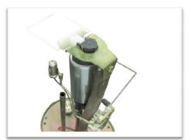
Refit the washer to the pump station assembly.
