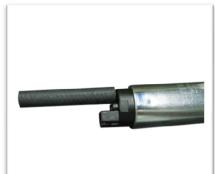
Use the mounting clips to fit the filter that was supplied to the Fuel Pump. Then attach the hose.
