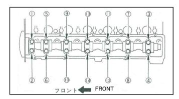
Start tightening the bolts from the left side of Cylinder No. 1, at TDC on the compression stroke. Then follow the numerical order.
