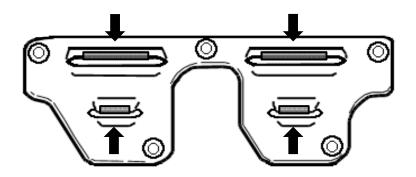
Make the required clearance of 1mm-1.5mm on the areas shown on the illustation on the left, to allow clearance for the Conrods. These are the areas where the Conrods will make contact during rotation.
