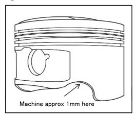
When using Tomei Pistons pre- August 2008, Stock pistons and some aftermarket pistons will need extra work to prevent the oil jets from making contact with the pistons.
