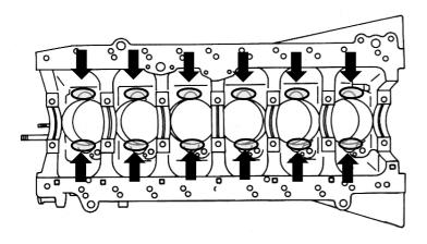
The marked areas as shown on the illustration on the left, shows the 12 points where the Conrods may make contact with the cylinder block. Process the required machining with a grinder to allow 1mm-1.5mm clearance when required. (shown with the mark)
