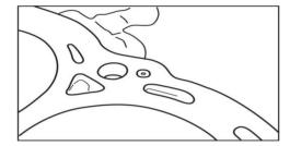
② Using a 5mm pin punch, depress the stock oil restrictor by 6mm.
