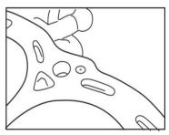
$\Phi$ 1.5mm restrictor installed.
