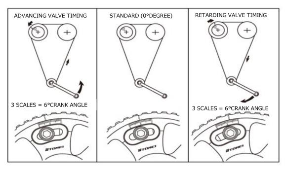
\* Each Scale on the KA cam gear is 2°(Crank angle 4°)
