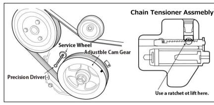
Insert at small screwdriver into the service hole of the timing gear case to push the ratchet of the chain tensioner open and you keep the driver there to keep it open.
