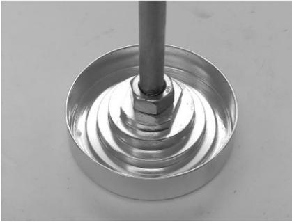
The upper spring support is stepped to accommodate the inner, middle and outer springs. Each spring should be seated on their respective step.
